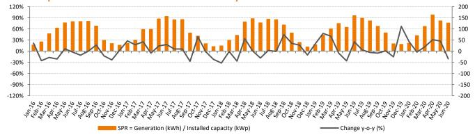
Specific Performance Ratio is a measure of efficiency which shows the amount of kWh generated per 1 kWp of installed capacity and enables the simple comparison of year-on-year results and seasonal fluctuations during the year.
