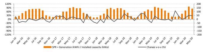
Specific Performance Ratio is a measure of efficiency which shows the amount of kWh generated per 1 kWp of installed capacity and enables the simple comparison of year-on-year results and seasonal fluctuations during the year.
